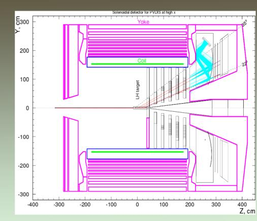
• Solenoid (from BaBar, CDF or CLEOII) contains low energy backgrounds (Moller, pions, etc) trajectories measured after baffles
